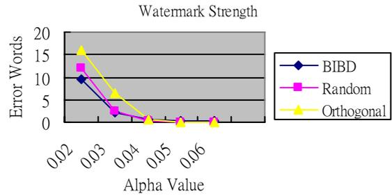
Fig. 4 Number of error words extracted by three coding approach in “Lena”
