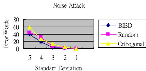
Fig. 6 Number of error words after Gaussian noise attacked ( $\alpha = 0.05$ )
