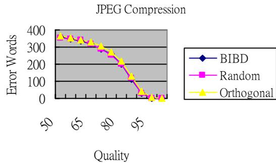
Fig. 11 Number of error words of three coding approach by JPEG compression
