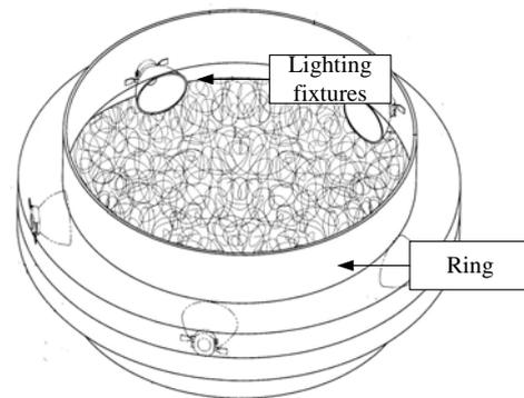
Fig. 3 The photocatalyst filter fixed in base
